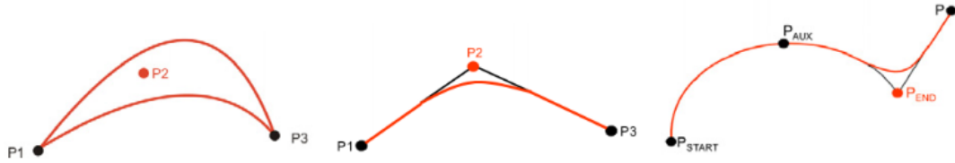
Figure 4. Approximate PTP, LIN, and CIRC positionings (adapted from KUKATM system software manual (KUKA AG, 2023)).
